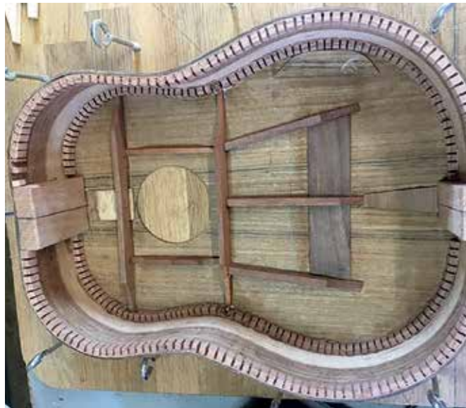
Caption: Inside the body showing the bracing
