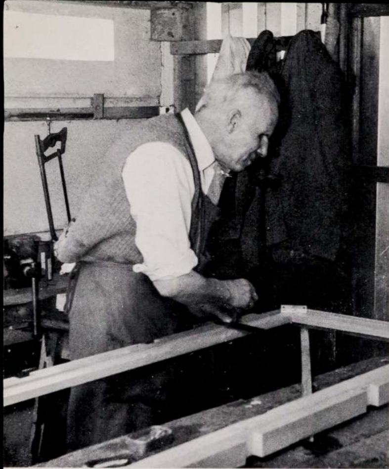
Leonard Parry making the frame for a fitted wardrobe in his garden workshop.
