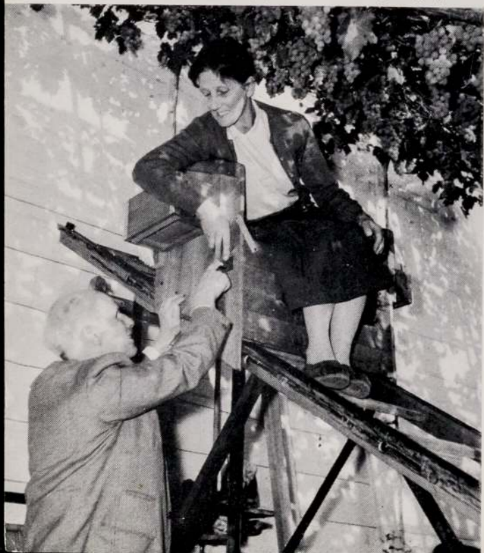
Explaining the use of a release device which enables the chair to slide up and down the ramp on the equipment for tending the grapevine.
