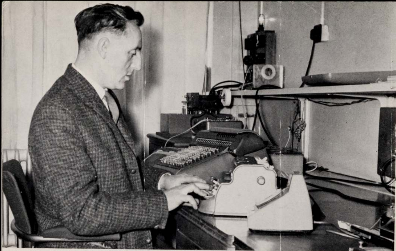
Ray Benson notes results obtained from his Braille desk calculator—seen behind his Braille writer.
