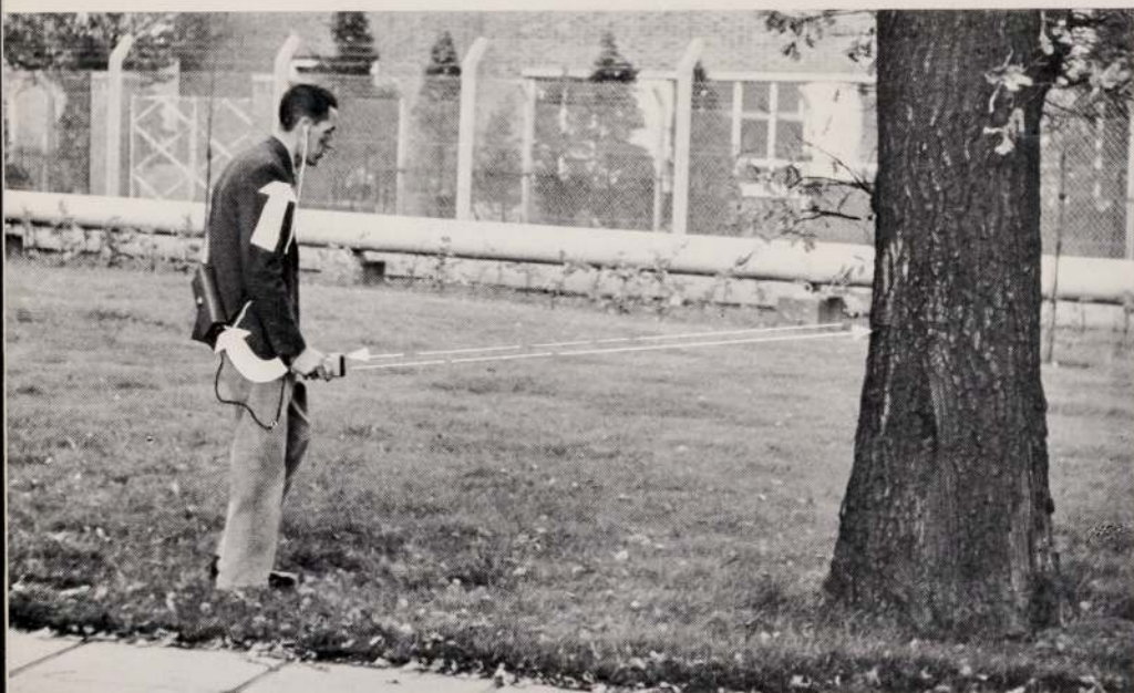
THE PRINCIPLE OF THE SONIC GUIDANCE AID: The small white arrows indicate the ultra-sonic signals from the transmitter in the probe and the echoes returning to the receiver. The large white arrows represent the audible tones from the aid passing to the ear of the user.
