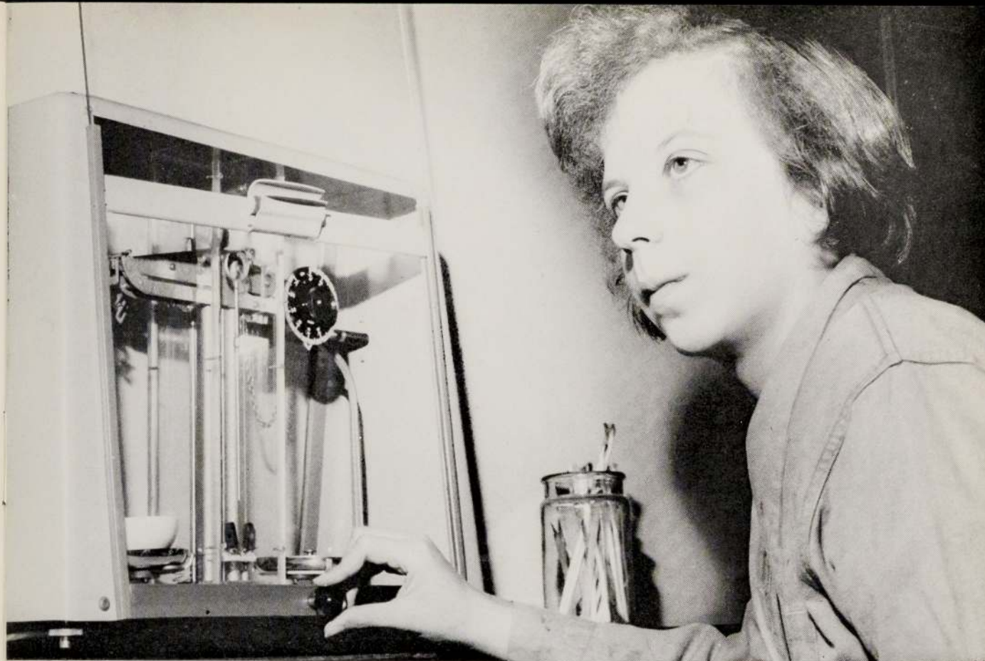
By using an adapted chemical balance, this student at Chorleywood College for girls with little or no sight can weigh chemicals accurately by touch and by sound.
