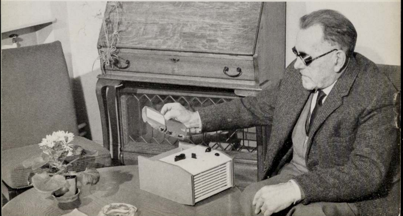
A subscriber to the British Talking Book Service for the Blind is about to insert the new 6½ oz. cassette into his machine.
