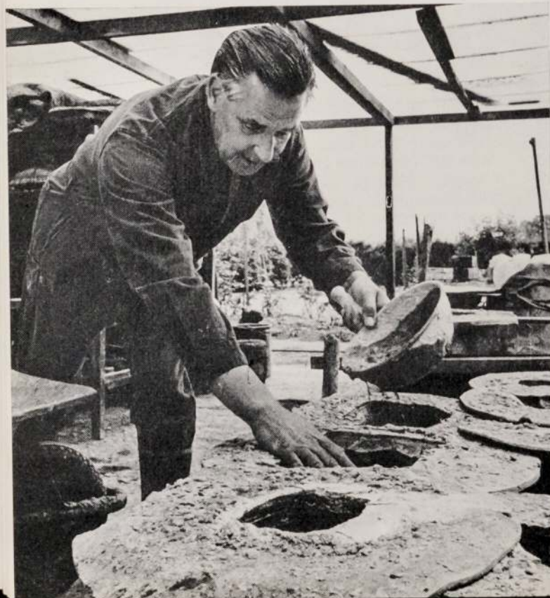
(Below) Pouring the concrete mix into a mould.
