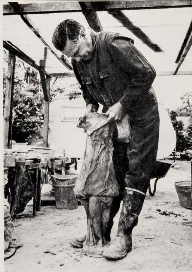
Moment of truth, and strain, as Reg peels off the rubber mould.
