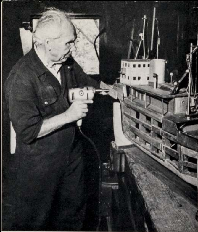
Bill Chamberlain using a template to drill port-holes.
