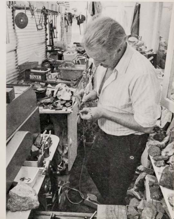
This high speed drill is controlled by means of a foot pedal.
