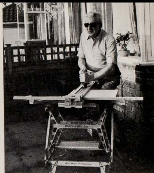
Peter demonstrates his 'cross-bow' jig for cutting large pieces of wood.
