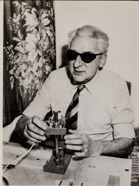
Using a miniature bench drill to make holes in a printed circuit board.
