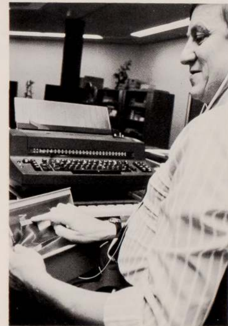
John uses Braille to code his file of magnetic cards which records the words typed.
