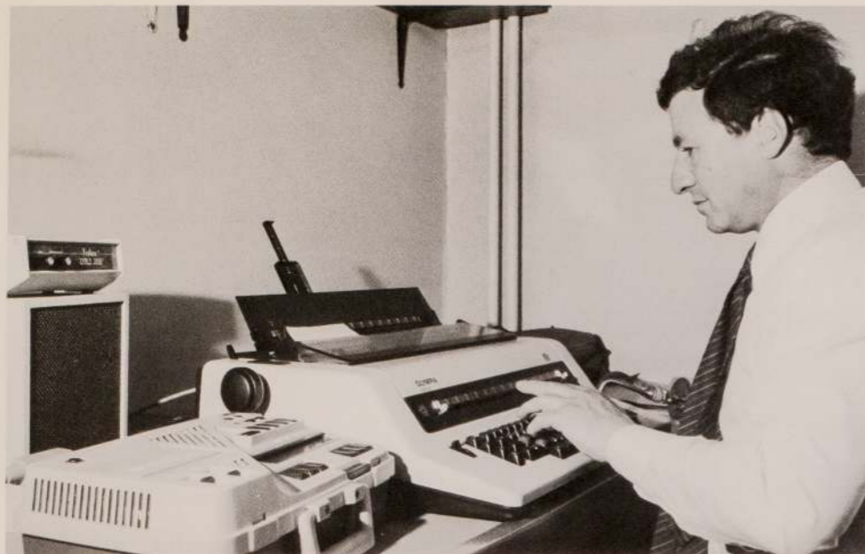
Ray Hazan's braille, print and spoken output systems. In the left foreground is the Versabraille and behind it the Votrax Type 'N' Talk unit with its loudspeaker. Ray is typing on the Olympia ESW 103 which also acts as a printer.
