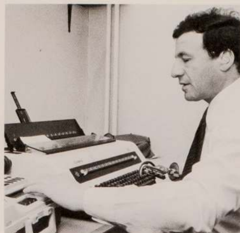
Checking what he has typed by means of the braille display on the Versabaille Ray can also listen to what he has written through the Type 'N' Talk — but this may not show up a spelling mistake.
