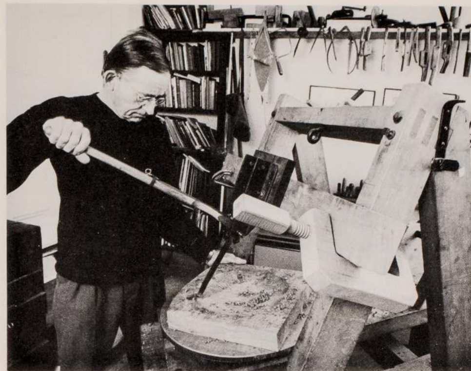
David Pye carving flutes with the device he invented. Photo: David Cripps.
