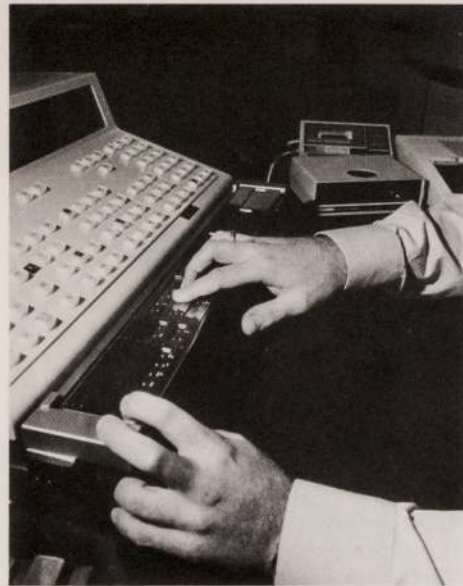
A close-up of the tactile indicator which reproduces the positions of the relevant light signals on the main board.
