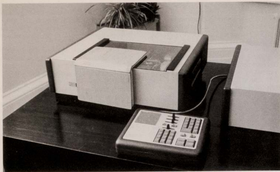
The three units of the Kurzweil Reading Machine: keyboard, scanner and (partly) electronic computer unit.
