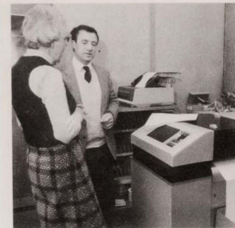
The output of the system is through the Braillo high-speed embosser, which produces a complete volume in about seven minutes.
