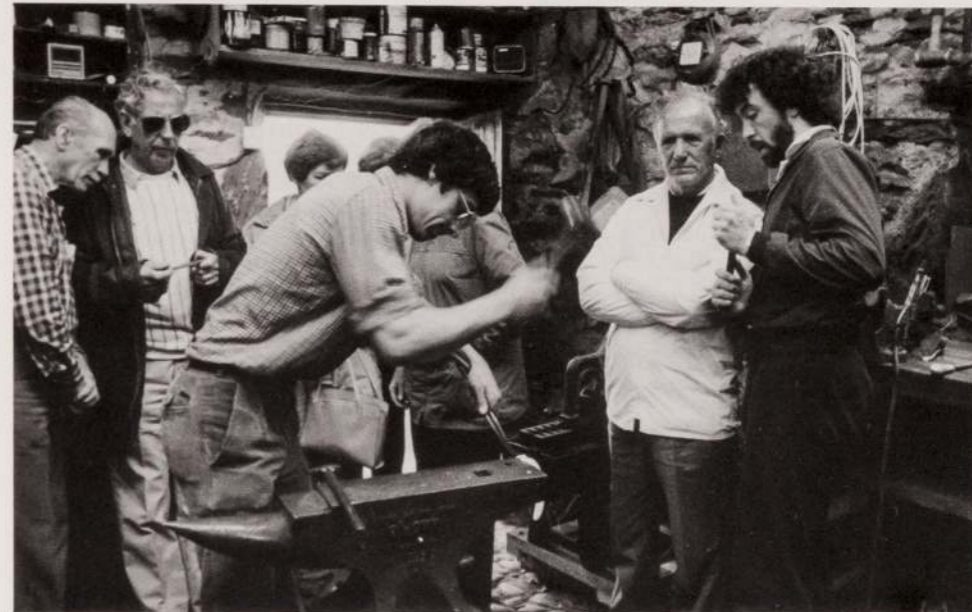
In Richard Ellis' smithy, the group watches him fashion a horse-shoe on the anvil.
