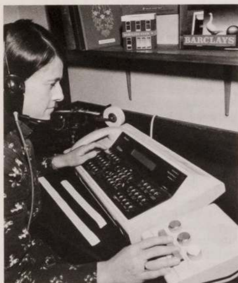
The Monarch switchboard system with voice synthesis unit attached.
