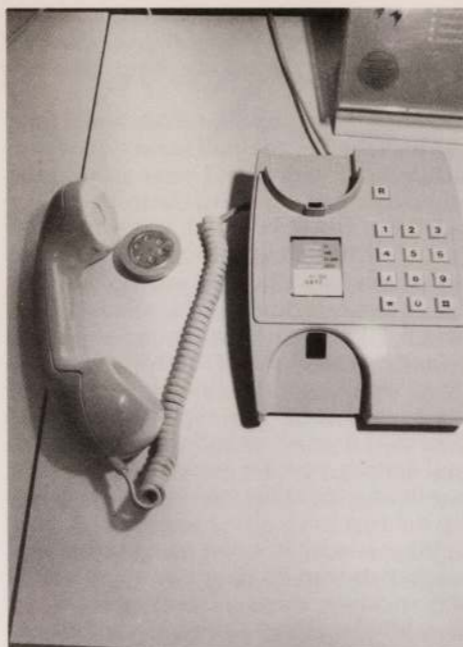
The inductive coupler which fits into the earpiece for hearing-aid users.
