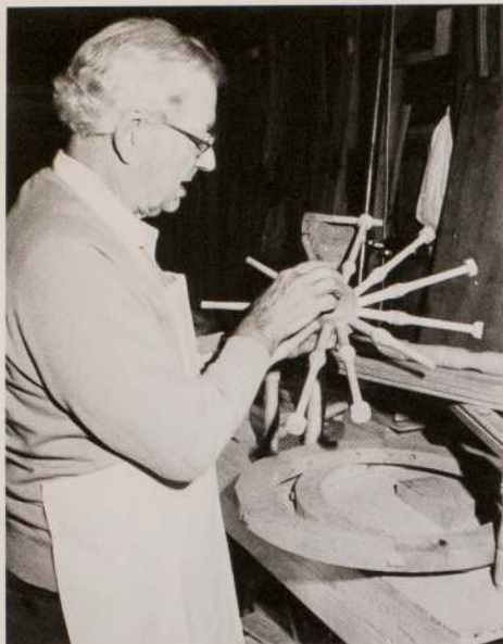
Assembling the wooden spokes in the split hub.
