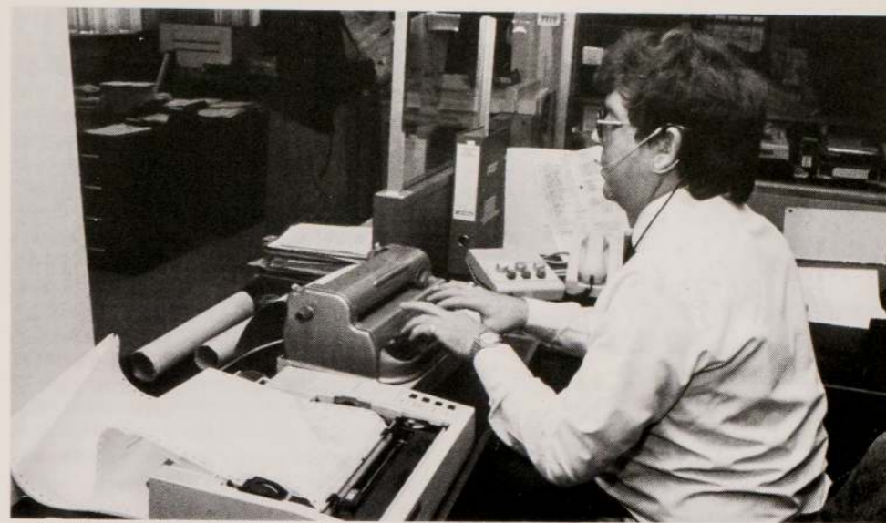
As Don Planner types in braille, a print version of his note is also produced.
