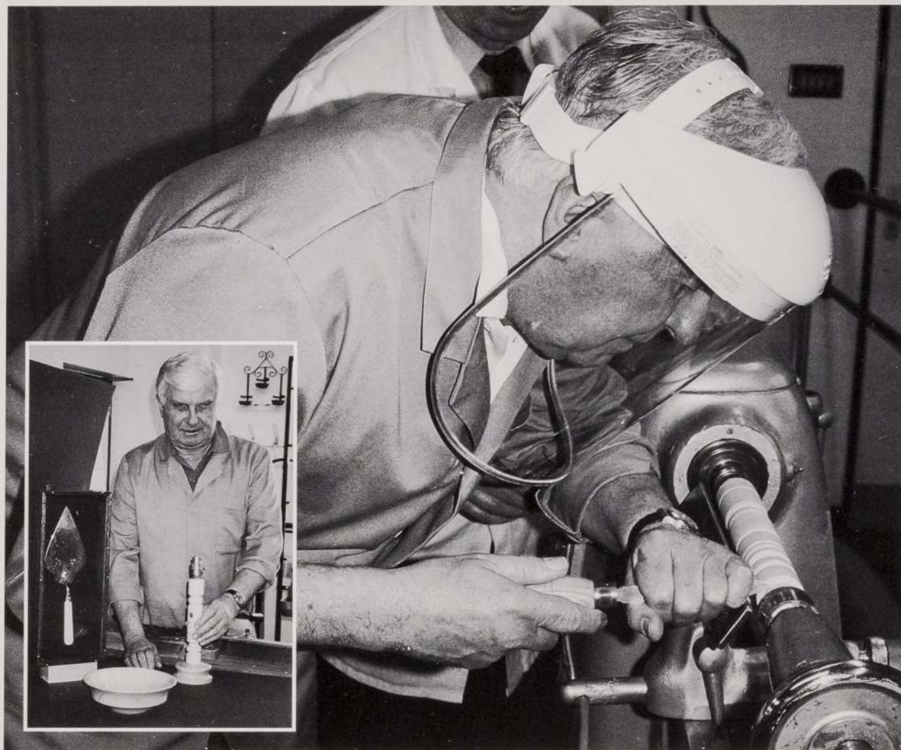
Steadying the chisel, Ted experimented with shaping the wood as it rotated at high speed on the lathe. Inset: Ted with a number of items he produced while on the course.
